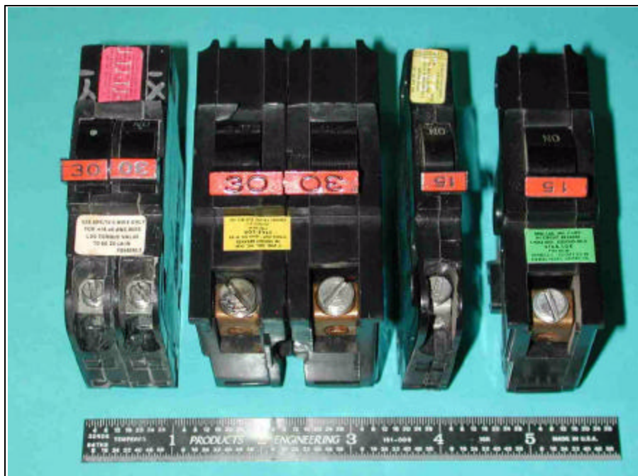
FIGURE 1 - REPRESENTATIVE SAMPLES OF HALF- AND FULL-WIDTH FPE STAB-LOK® CIRCUIT BREAKERS (left to right: 1/2-width double pole, full-width double pole, 1/2-width single-pole, full width single-pole) Note that the color and style of the handle varied over the years.
